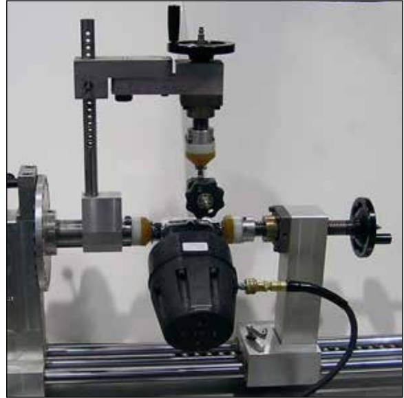
Leak and Shell Test
